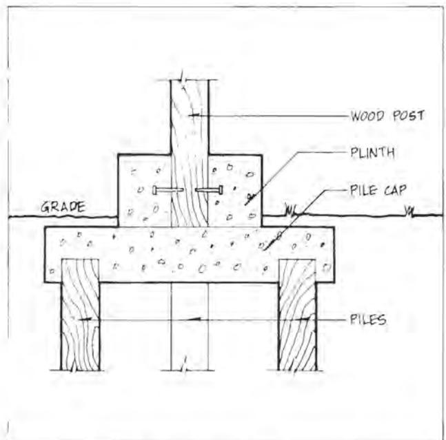
Figure 4.8. Post/Pile Foundation
