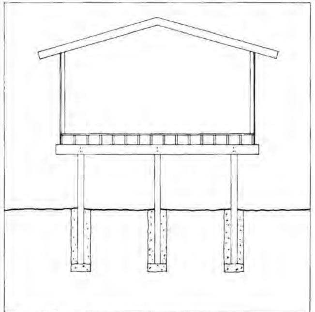
Figure 4.28. Platform Construction
