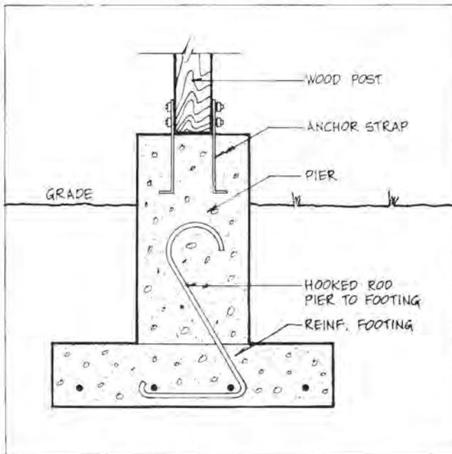
Figure 4.9. Post/Pier Foundation
