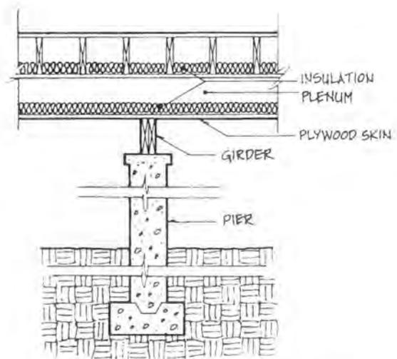
Figure 4.53. Double-Insulated Floor Plenum, Pier Foundation
