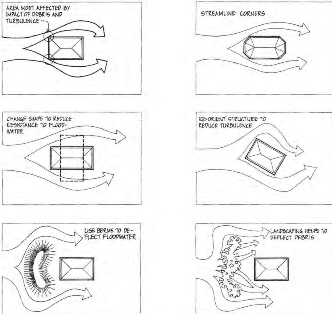
Figure 2.6. Site Design to Reduce Flood Hazards
