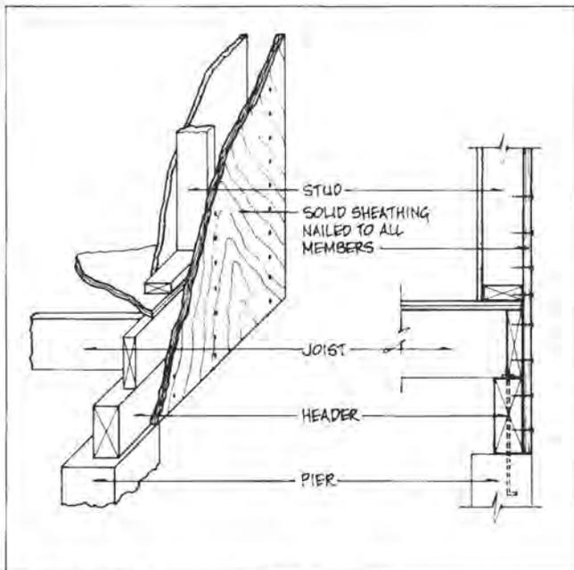
Figure 4.45. Plywood Anchorage
