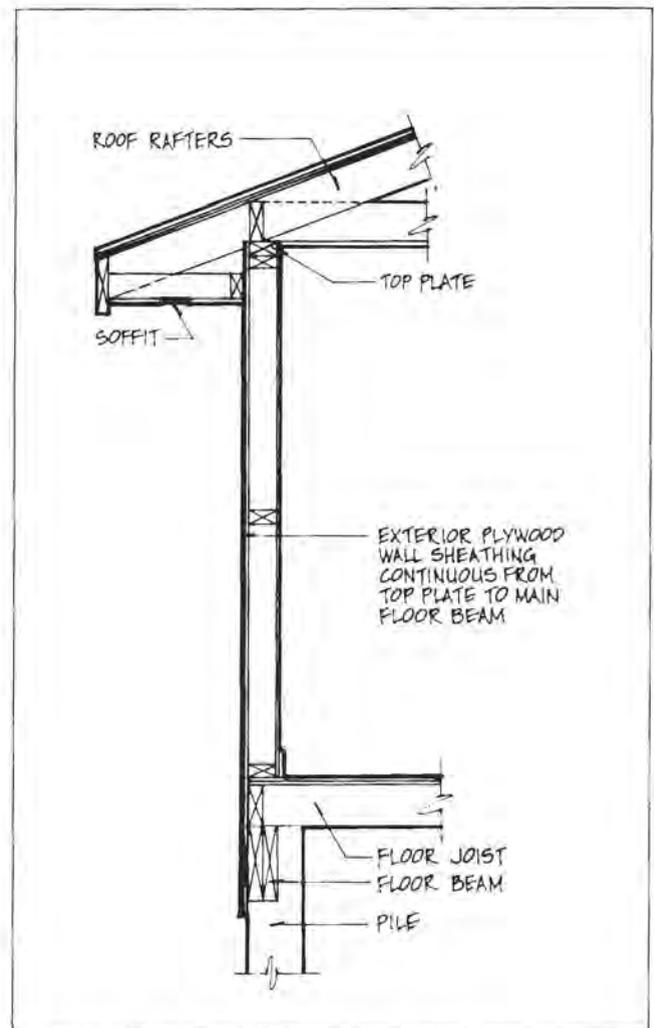
Figure 4.46. Wall Sheathing Tie from Roof to Ceiling.
