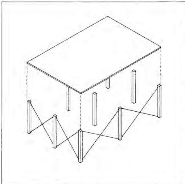
Figure 4.22. Diagonal Bracing
