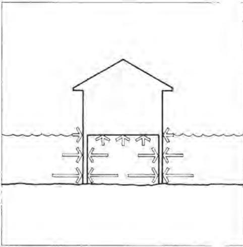
Figure 2.1. Hydrostatic Forces
